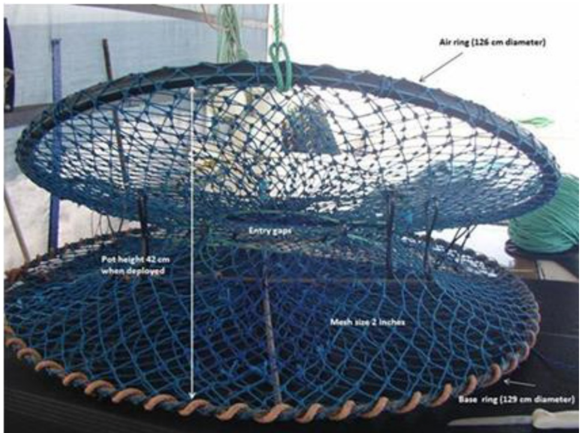
Figure 37: Example of a collapsible crab trap (showing an entry gap to minimize bycatch) used in the Shark Bay Crab Managed Fishery. Taken from (DPIRD 2020).
